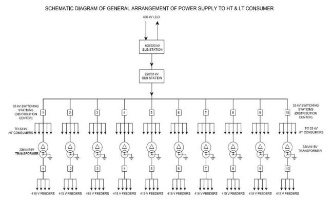
Proposed installed capacity of each 220KV/33KV Substation: 3x80MVA= 240MVA. Total installed capacity of all 220KV/33KV Substations = 16x240 + 720 (Incoming SS) = 4560 MVA i.e. 1.56 times the assessed demand of Amaravati City. Proposed 400KV/220KV, 220KV/33KV Substations & 33KV Switching Indoor GIS Substations are located across the city for distribution of power to the end consumer as shown in the map and SLD.
