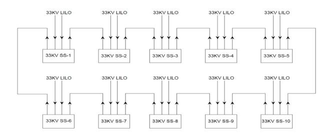
NOTE:-1. LINE IN LINE OUT ARRANGEMENT FOR 33KV INCOMING FEEDERS FROM 220/33KV SOURCE.
