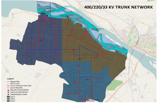
During development in a phased way, Cable Trench routings to be planned in such a manner to utilize the same duct, even if the source of power supply is changed to a **particular** area from the in-service Substation to a new substation
